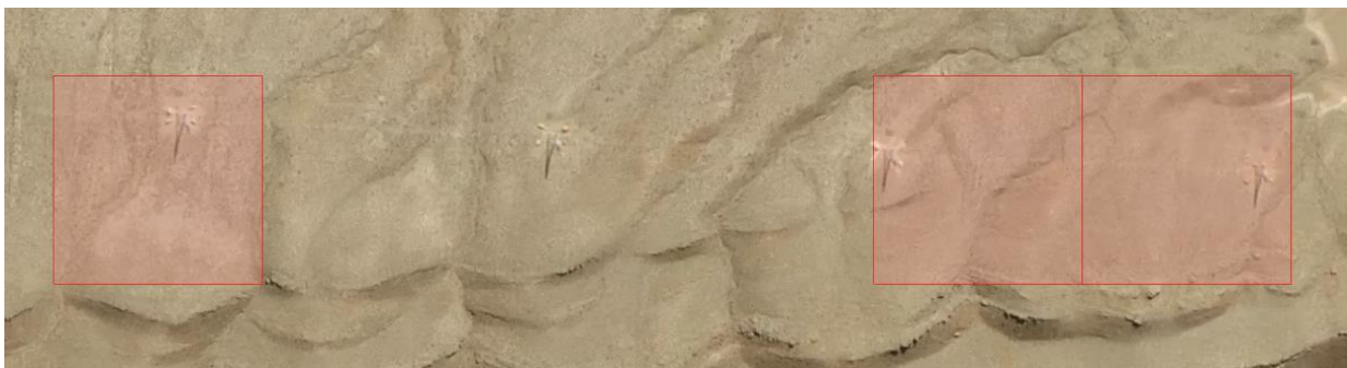
Figure 3. Find HV towers in satellite imagery with ML. The goal of the ML component was to detect as many HV towers as possible; here three of four. With this overlay, our Data Team could start tracing from these high-priority locations and fan outward to map the entire HV grid.
