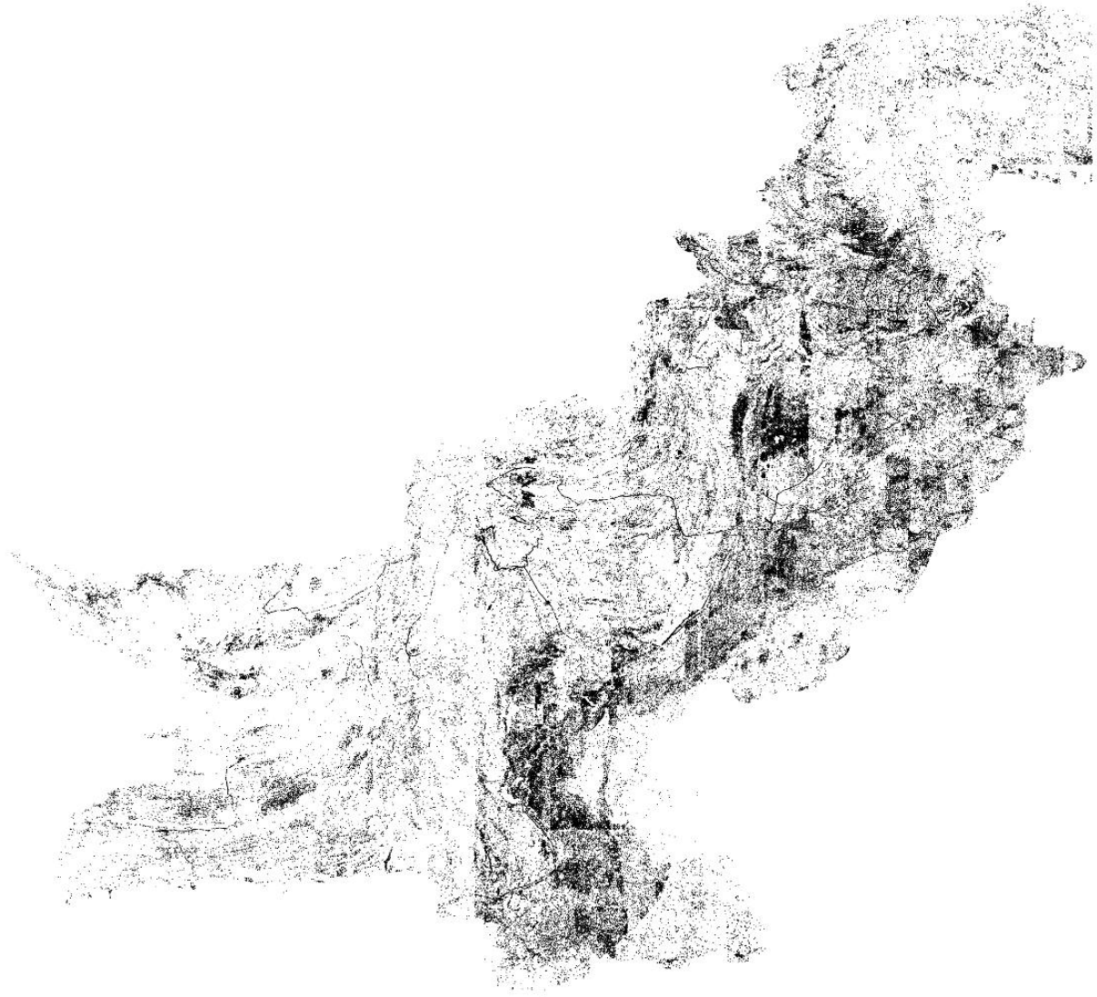
Figure 13. Country-wide prediction map in Pakistan. Black dots correspond to locations where the model predicts a HV tower was present. In the mountainous desert region of Pakistan, the model performed relatively well. In the Eastern agricultural region, the model predicted many more false positives as there were no any training data obtained from that region.
