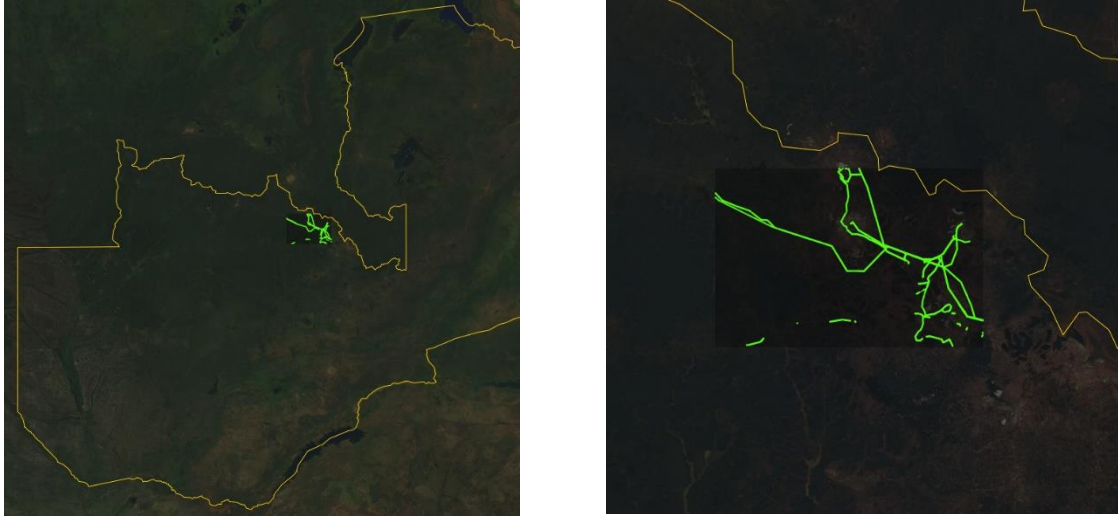
Figure 7. Training region for Zambia. Green features represent HV infrastructure included in the training data. There are some broken lines as HV infrastructure was only included if it was visible on the Digital Globe Vivid layer.
